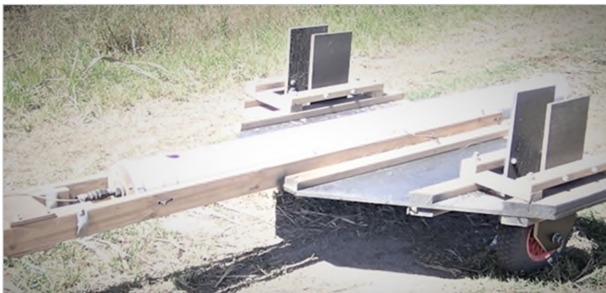
Figure 20: EMI trailer, showing instrument housing, cabling and out-rigger wheel assembly
