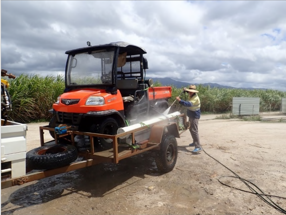
Figure 22: Pressure washing survey equipment
