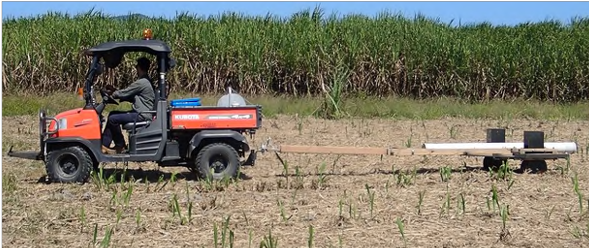
Figure 2: The DualEM instrument being towed in the field by an RTV
