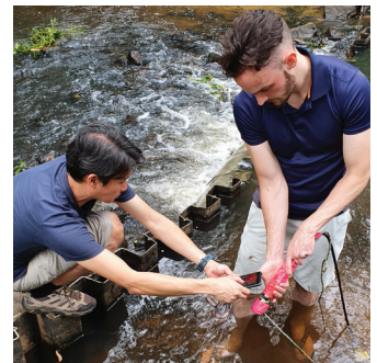
Implementation of nitrate sensor for 1-month Limited-Field Trial
