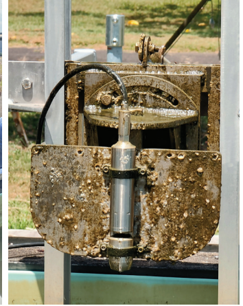
Nitrate sensor checks completed at the Rocklea Hydrographic Support Unit
