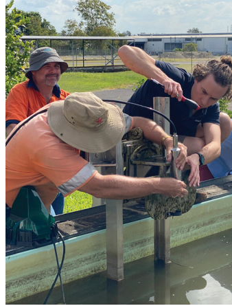
Installation of nitrate sensor at the Rocklea Hydrographic Support Unit
