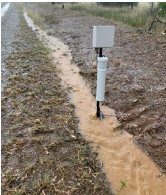
Figure 4: LGAQ sediment sampler (left) and inverse relationship between sediment concentration and vegetation cover (right).
